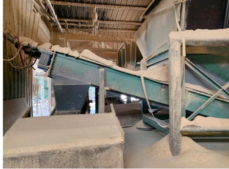
Constantly monitor temperature of machinery and motor bearings to prevent combustion from dust buildup.
