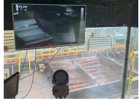
A FLIR thermal imaging camera is installed outside the control room to "see through" steam - preventing blockages in a log vat.
