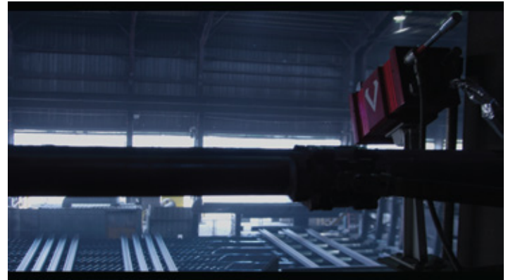
Monitor processes using ViperVision software, which provides both visual and thermal data.
